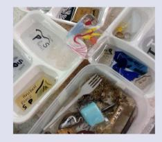
I tested materials in Polyoptic resin to ensure the heat process & chemicals did not distort or melt plastics, bleed inks, affect colours, or an array of media.
