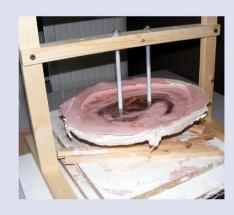
In order to fix the pieces on the wall, 2 lengths of steel threaded rod with nuts and washers for strength are embedded into the resin mould during casting.
